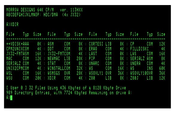
Fig 2. GMD128 splash screen followed by CP/M directory listing. GMD128 looks like a typical "green-screen" terminal of the 70's-80's period, in particular it will default to be a terminal which acts very similar to Televideo 920/ Soroc 120/ ADM3A terminals.
